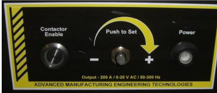
Figure 3-2, X-HW 200 Controls Cluster
