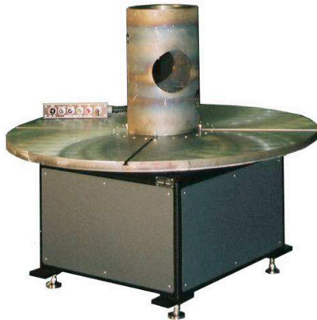
MTT-1000 Precision 1 Ton Motorized Turn Table
