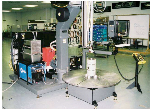
MTT-1000 used on Advent Bore Cladding System
