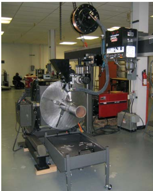
LTC track and carriage with SAW weld head over a PZT-1000 tilting positioner
