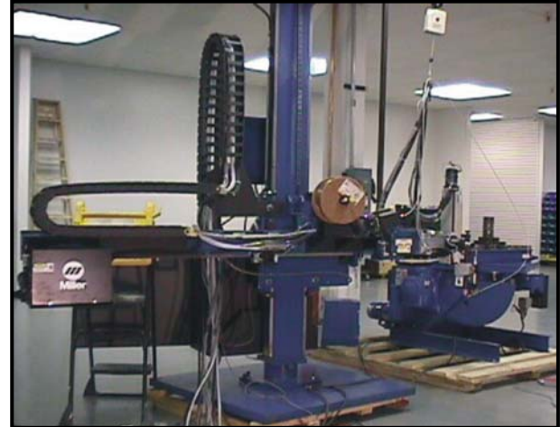
CBM-S-2x2 with GTAW and Positioner Puget Sound Naval Shipyard
